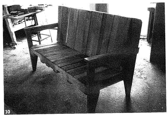
& Attach the arms (E). To create the arms (E), I installed a board on each side of the seat, attaching them to the side stretchers (D). It created a comfortable armrest as well as a good place to set a beverage.
